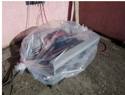
Fig.2. Electric motor windings prepared to be tester in explosive mixtures
