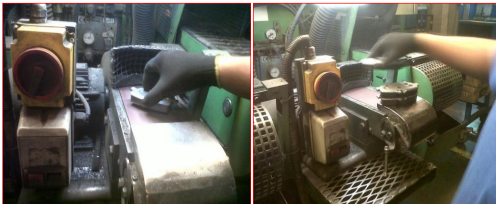
Fig.13. Projection of dust mix in the eye, particles carried by the air currents to the abrasive belt, dropping-jumping pads
