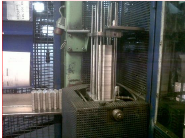
Fig.12. Machine parts in motion - hand grip when placing the plates in the magazine.
