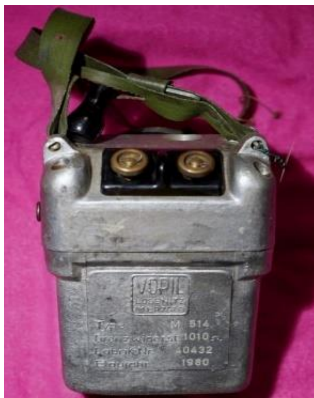
Fig.1. Vopil M514 Blaster machine
