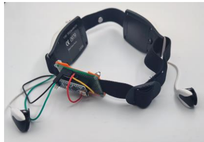
Fig.2. MindFlex neural headsets after hardware upgrades
