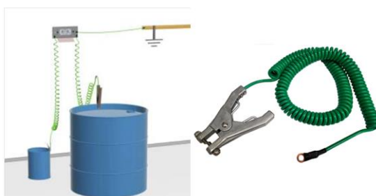
Fig. 3. Static Grounding Clamp capable of breaking through coatings, product deposits and rust to ensure a good electrical connection to process equipment
