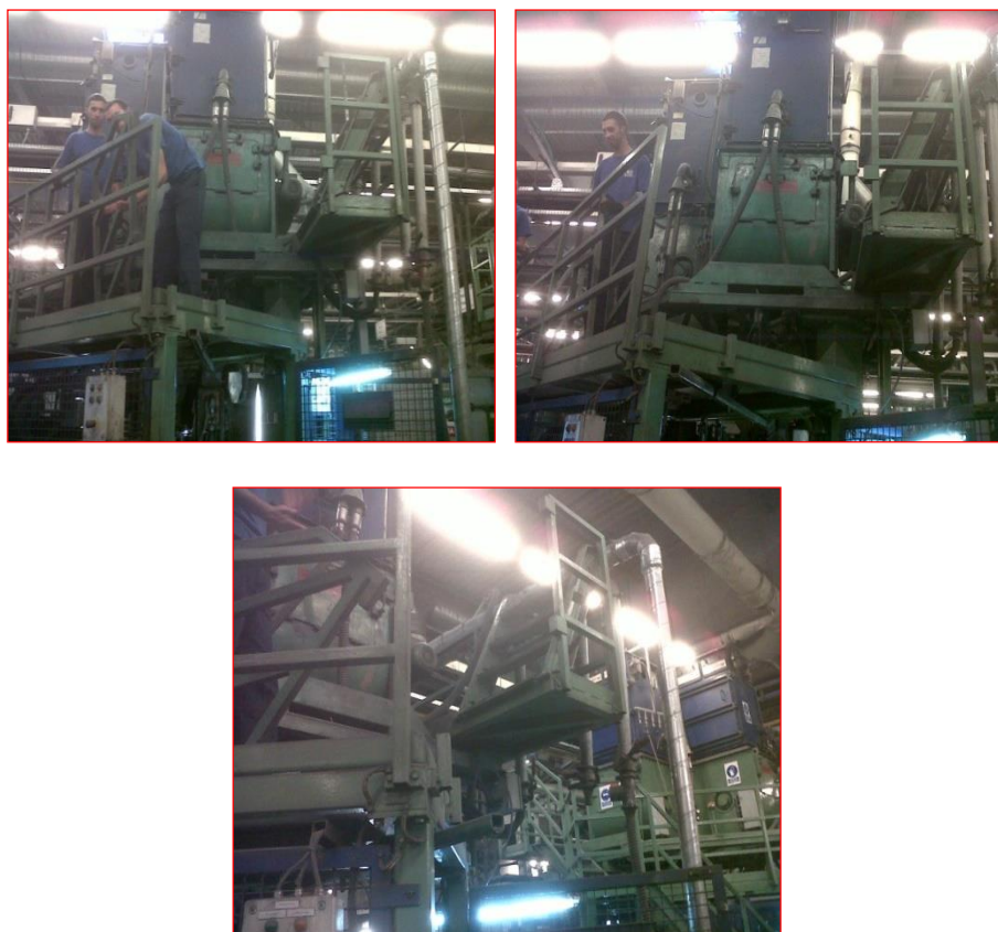
Fig.14. Falling from a height due to imbalance, slipping, tripping – when checking the level of mix in the mix in the hopper, when manually loading and emptying the hopper
